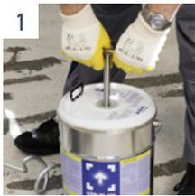
**1** Punch the plastic closure and floor of the cover insert of the combination pack several times with a strong metal punch (or screw driver). Do not forget to wear protective clothing!
