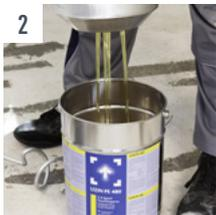
**2** Allow hardener liquid to run completely into the resin container.
